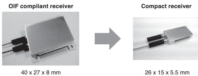
Fig. 7. Receiver package comparison
