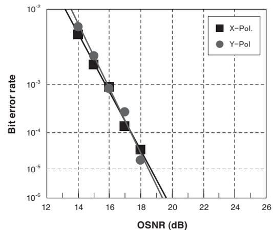
Fig. 13. BER vs. OSNR curve
