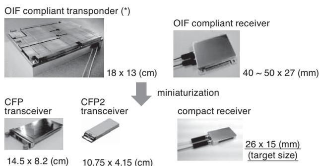
**Fig. 1.** Size of transceivers and receivers
