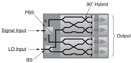
Fig. 2. Block diagram of coherent receiver
