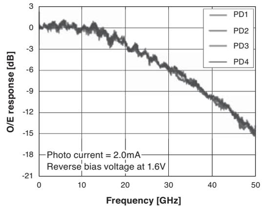
Fig. 4. Optical/Electrical response
