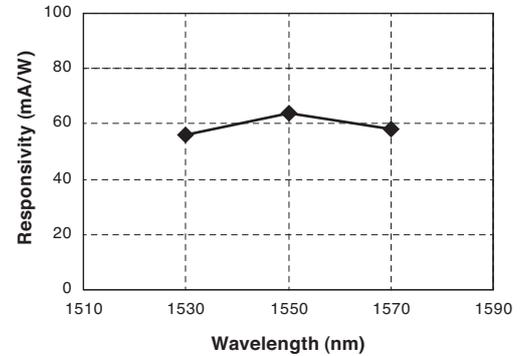
Fig. 8. Responsivity wavelength dependence
