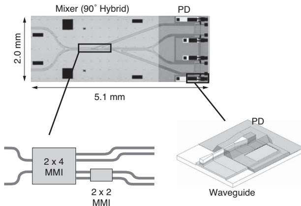
Fig. 3. InP-based mixer with integrated PD
