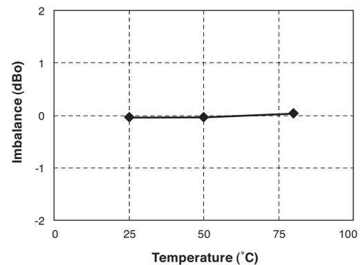
Fig. 9. Imbalance temperature dependence
