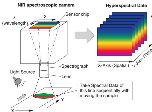
Fig. 1. Processing of Hyper spectral data with NIR spectroscopic camera
