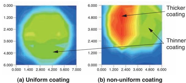
Fig. 5. Image of thickness of magnesium stearate coating (This figure is result of collaborative work with prof. Ozaki group in Kwasei Gakuin Univ.)
