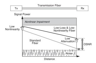
Fig. 1. Schematic of OSNR improvement by low attenuation and low nonlinearity of fiber
