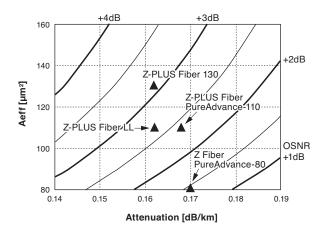
Fig. 5. Relative OSNR normalized to that for SSMF in a 1500km-reach transmission link with 80km-span
