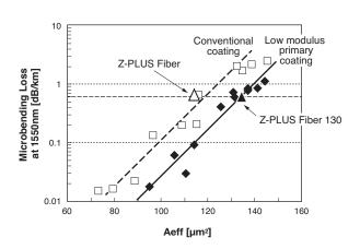
Fig. 3. Microbending loss for fibers with low Young's modulus primary and conventional coatings
