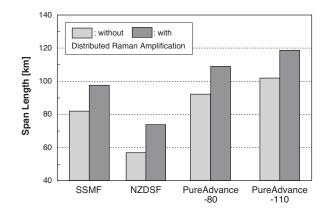
Fig. 6. Maximum span length for a 1500km transmission link with 100 Gb/s DP-QPSK format
