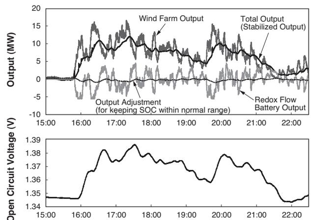
**Fig. 9.** Output waveform stabilized by a redox flow battery system
