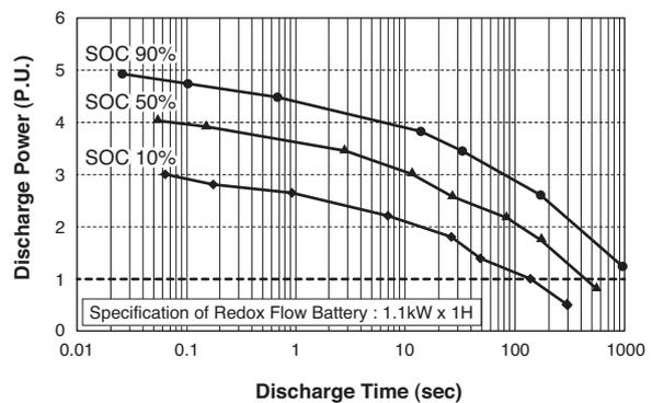
Fig. 6. High power characteristics of a redox flow battery
