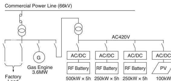
**Fig. 13.** The circuit configuration of a megawatt-class electric power generation/storage system
