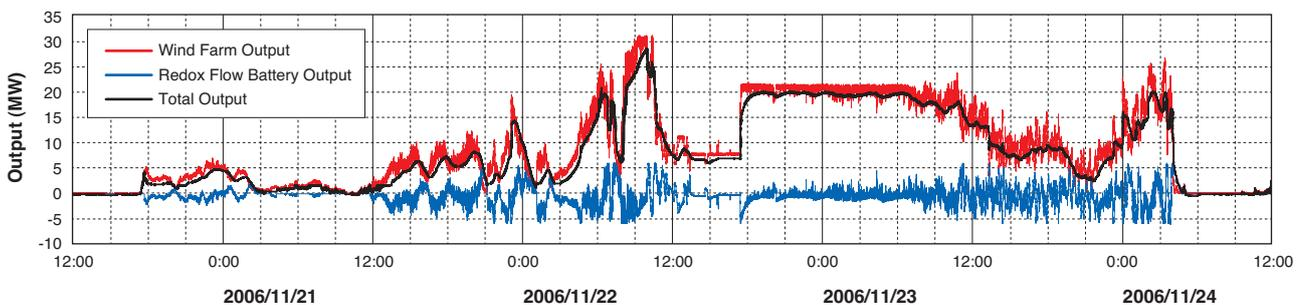
**Fig. 12.** Example of wind farm power output stabilization
