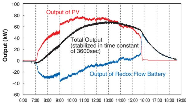
Fig. 14. Stabilizing solar power output operation
