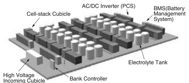
**Fig. 10.** The layout of 6 MWh redox flow battery system
