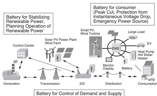
Fig. 1. Expected applications of batteries
