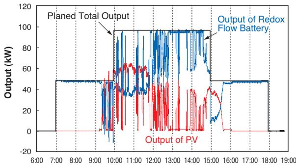
Fig. 15. Planned operation of the solar power output
