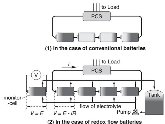
Fig. 4. Schematics of SOC variability between series-connected batteries
