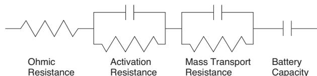
Fig. 7. Single equivalent circuit of a redox flow battery
