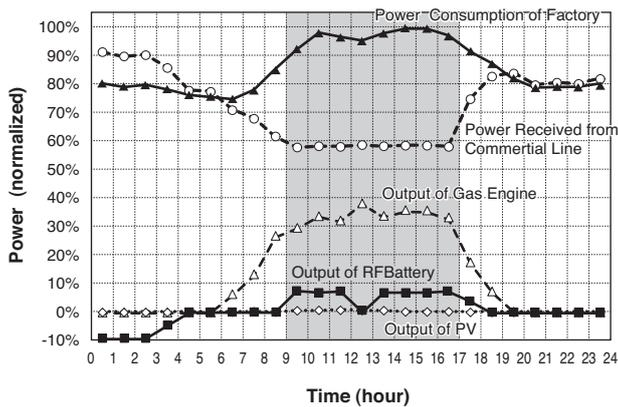
Fig. 16. Peak-cut operation
