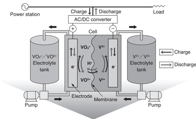
Fig. 2. Principle and configuration of a redox flow battery
