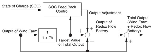
**Fig. 8.** Flowchart for stabilizing the fluctuations in output of a wind farm using a redox flow battery system
