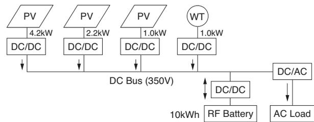
Fig. 17. The circuit configuration of the micro grid system
