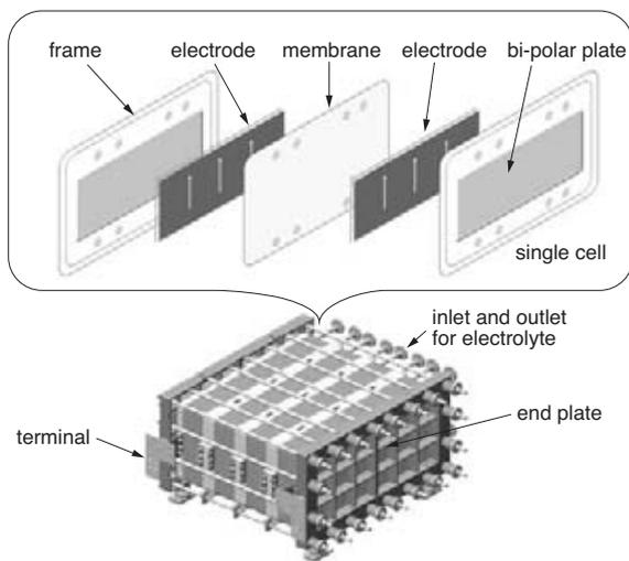
Fig. 3. Typical structure of a cell stack
