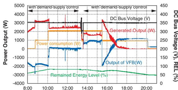
Fig. 18. Demand/supply control by 10 kW redox flow battery system
