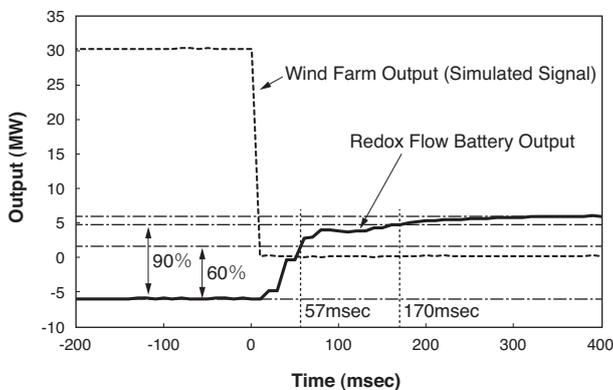
Fig. 5. The measurement results of response time of a 6 MW redox flow battery system
