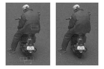
Photo 4. Example of the result of plate detection Left: without preprocess Right: with preprocess
