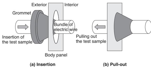
Fig. 1. Schematic illustration of test
