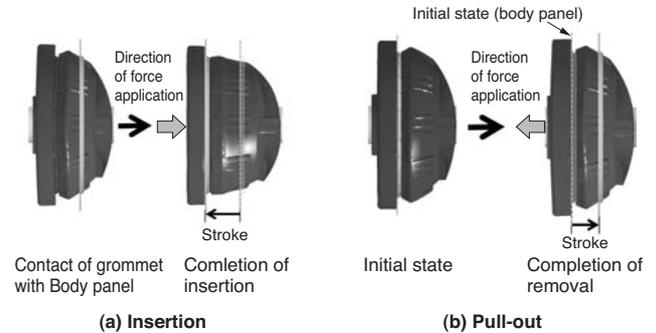
Fig. 2. Definition of insertion and pull-out forces and strokes
