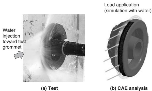
**Fig. 14.** Testing and analysis of grommet simulating car washing
