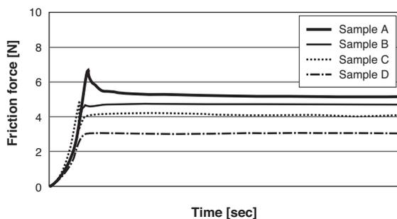
(b) Difference in frictional force (contact between rubber material and body panel)
