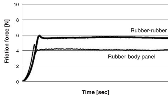
Fig. 7. Comparison of frictional forces
