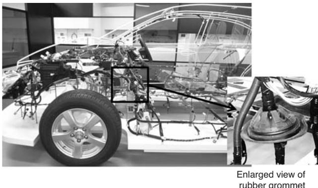
**Photo 1.** Automotive wiring harnesses
