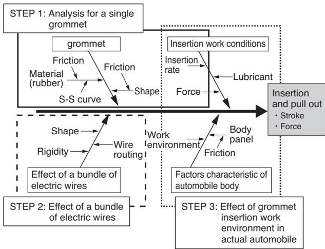
Fig. 4. Cause-Effect Diagram (insertion and pull-out)
