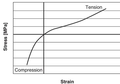
Fig. 6. S-S curve of rubber material
