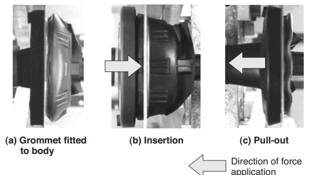
Fig. 3. Deformation of grommet (b and c show deformations under peak loads.)
