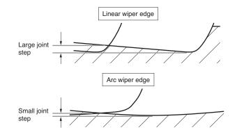
Fig. 4. linear and arc wiper edges
