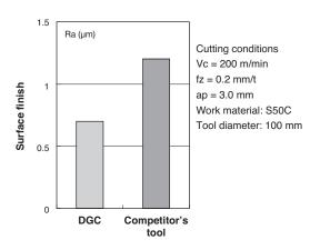
Fig. 5. Quality of machined surface
