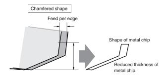
Fig. 9. Shape of metal chip for chamfered chip breaker
