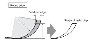
Fig. 8. Shape of metal chip for chip breaker with round edge
