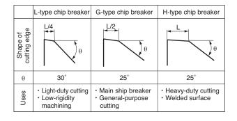
Fig. 6. Chip breakers
