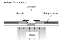
Fig. 4. Thermal conductivity measurement
