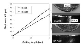
Fig. 2. Tool failures in ferrous PM machining
