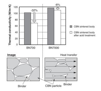
Fig. 5. Thermal conductivity of CBN compact
