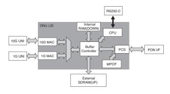
Fig. 3. Block Diagram of Communication LSI for ONU
