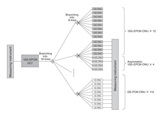
Fig. 5. Actual Equipment Verification Environment for 128 ONU System
