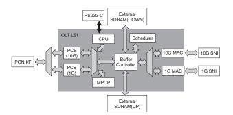
Fig. 2. Block Diagram of Communication LSI for OLT
