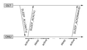
Fig. 4. Power-saving Control Protocol Flow
