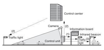
Fig. 1. System configuration
