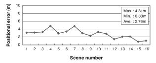
Fig. 5. Positional error of high-definition camera
