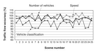
Fig. 4. Traffic flow measurement accuracy of NTSC camera
