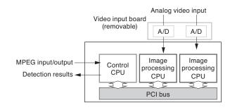
Fig. 3. Processing board configuration
