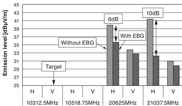
Fig. 11. Comparison of the emission level at the various frequencies
