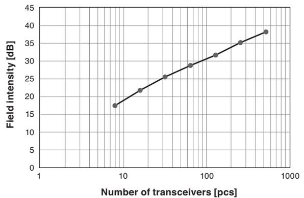
Fig. 5. Relationship of the field intensity and the number of noise source
