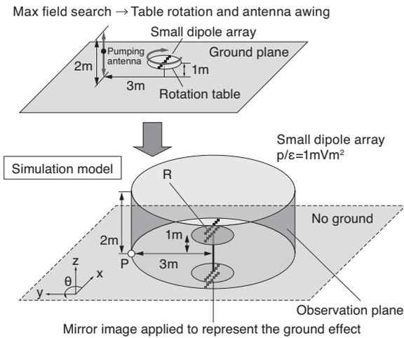
Fig. 3. Simulation model
