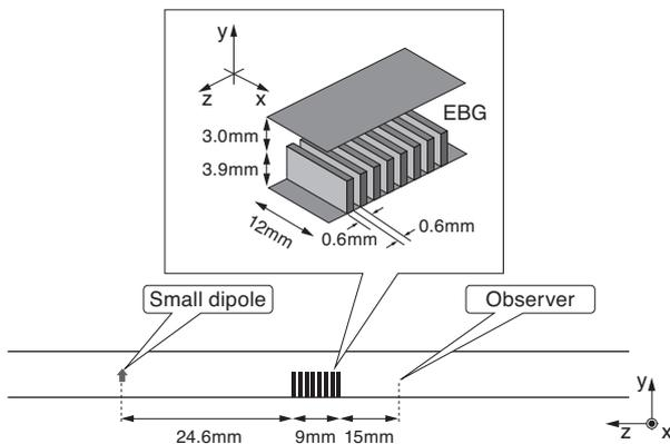
**Fig. 8.** Simulation model for EBG
