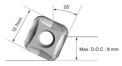
Fig. 1. DNX Series Indexable Insert Size and Cutting Edge Specifications
