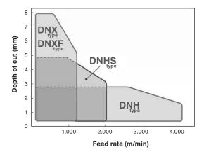
Fig. 6. Application Range of DNX-Series Cutters
