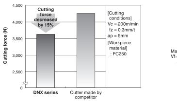
Fig. 3. Cutting Force Comparison
