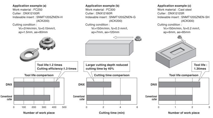
Fig. 8. Application Examples of DNX-Series Cutters
