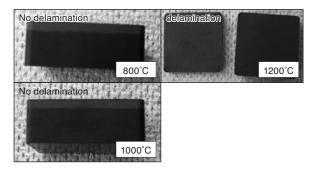
Photo 5. Appearance of sintering in low temperature
