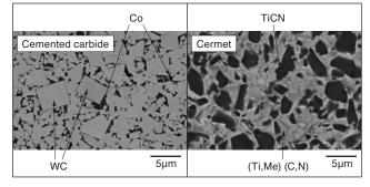
Photo 1. Micro structure of SEM
