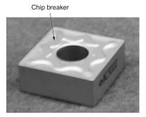
Photo 2. Cutting tool of cemented carbide
