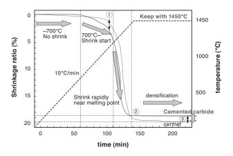
Fig. 3. Comparison of shrinkage behavior
