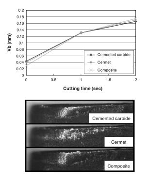
Fig. 4. Cutting performance of wear resistance
