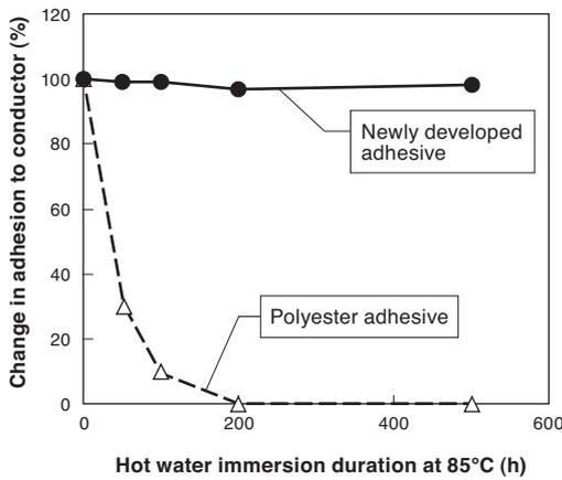
Fig. 5. Variation over time in adhesive strength
