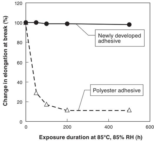
Fig. 4. Variation over time in mechanical properties of adhesive
