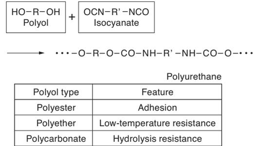
Fig. 6. Types and structures of anchor coatings
