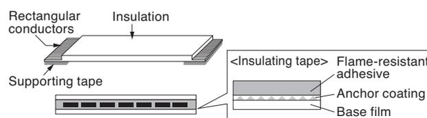
Fig. 1. Structure of flexible flat cable
