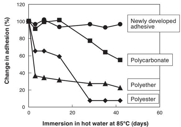
Fig. 7. Hot water resistance comparison of anchor coatings
