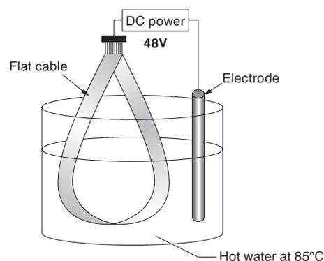
Fig. 2. Hot water test method
