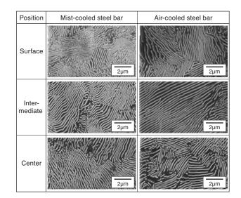
Photo 3. Pearlite Lamella Structures by SEM
