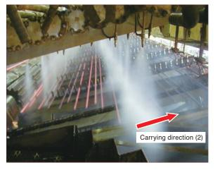
Photo 1. External Appearance of Steel Bar Mist-Cooling System in Operation
