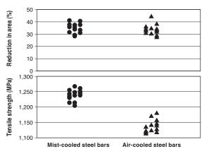
Fig. 6. Mechanical Properties of Steel Bars
