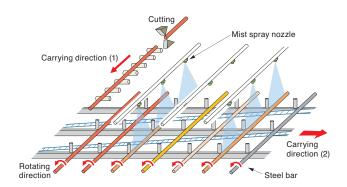
Fig. 4. Schematic Illustration of Steel Bar Mist-Cooling System
