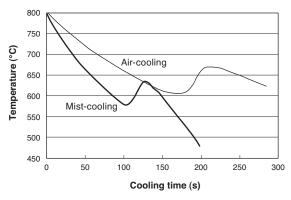
Fig. 5. Cooling Curve for Steel Bars
