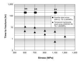
Fig. 1. Delayed Fracture Properties Comparison between Pearlite Steel and Tempered Martensite Steel
