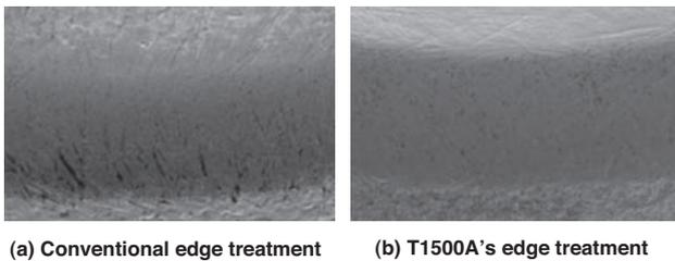
**Photo 1.** Comparison of the conventional and T1500A's edge treatment
