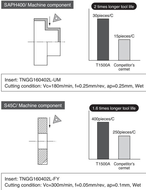
Fig. 8. The application of G-class T1500A
