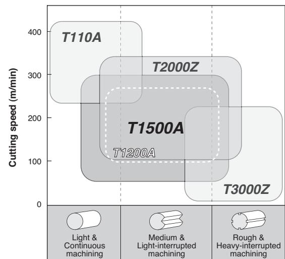
Fig. 1. The lineup of various cermet materials for steel turning
