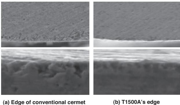
**Photo 2.** Comparison of the states of conventional cermet edge and T1500A's sharp edge
