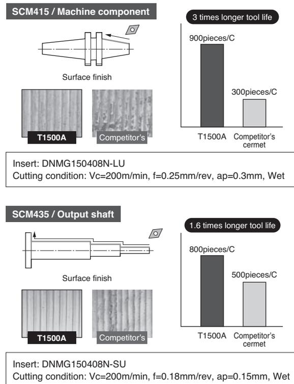
**Fig. 7.** The application of M-class T1500A
