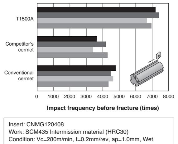
**Fig. 5.** Evaluation results on fracture resistance under interrupted machining
