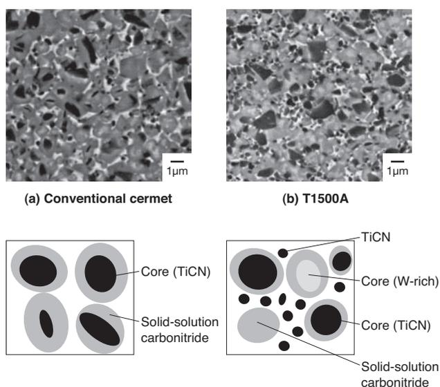
Fig. 2. Structures of the conventional cermet and T1500A
