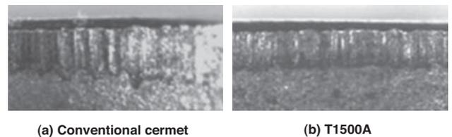
**Photo 3.** Edge states after wear resistance test
