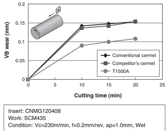
**Fig. 4.** Evaluation results on wear resistance
