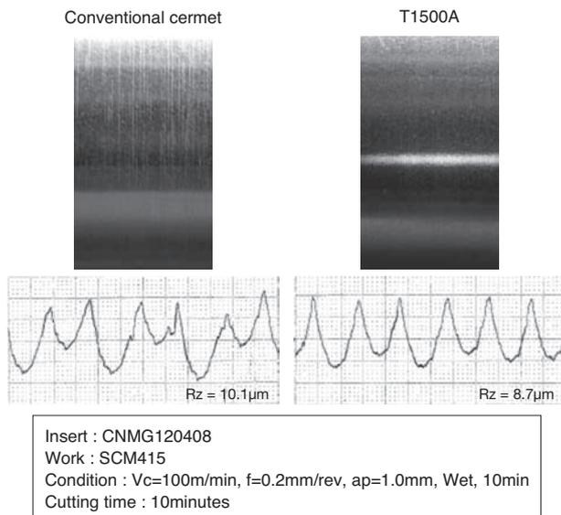
Fig. 6. Evaluation results on finished surface
