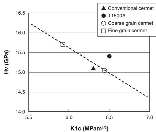
Fig. 3. Relationships between fracture toughness (k1c) and Vickers hardness (Hv)
