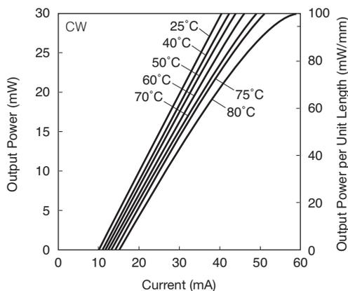
Fig. 5. Temperature dependence of  $L$ - $I$  characteristics (Improved  $L = 300 \mu\text{m}$  LD, CW operation)
