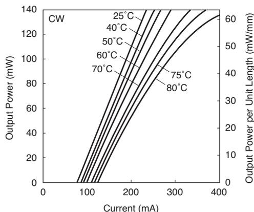
Fig. 2. Temperature dependence of  $L-I$  characteristics ( $L = 2200 \mu\text{m}$  LD, CW operation)
