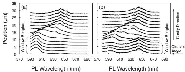
**Fig. 1.** PL spectra profiles of Zn-diffused window region
