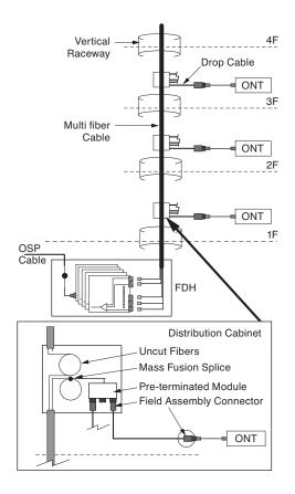
Fig. 2. Conventional optical solution (2)
