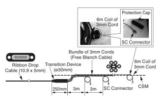
Fig. 7. Cable configuration for small MDU
