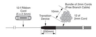
Fig. 4. Cable configuration for large MDU
