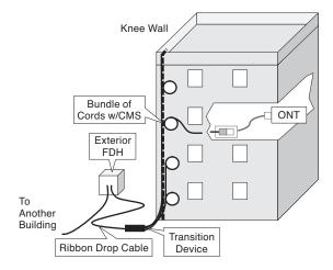
Fig. 6. Cable network for small MDU
