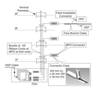
Fig. 3. Cabling network for large scale MDU
