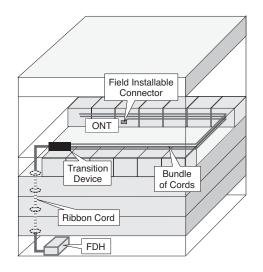
Fig. 5. Cabling network for middle scale of MDU
