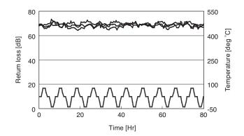
Fig. 7. Return loss properties of field assembly angled polishes SC connectors for 0.9 mm fiber at heat cycle test
