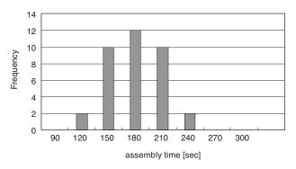
Fig. 6. Working time of connectors for ø0.9 mm fiber (MM50 type) by amateur worker
