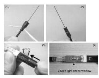
Photo 2. Outline of assembly procedure of field assembly connector for ø3 mm cord
