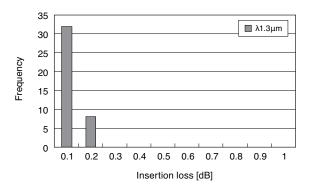
Fig. 5. Insertion loss distribution of assembled connectors for Ø0.9 mm fiber by amateur worker
