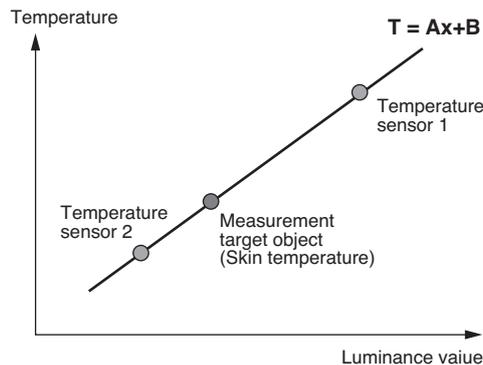
Fig. 7. Calculation method of absolute temperature
