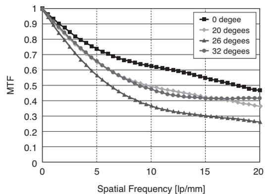
Fig. 4. MTF evaluation results for the developed wide-angle lens
