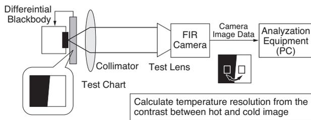
Fig. 5. Test system of temperature resolution performance
