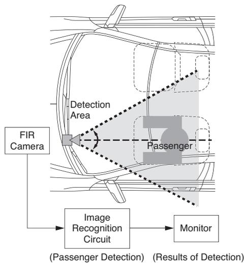
**Fig. 1.** Newly developed automobile occupant detection system using FIR camera
