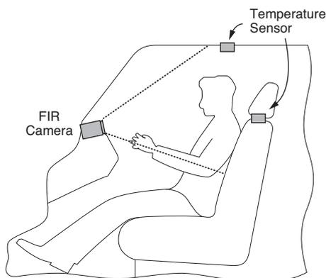
Fig. 6. Absolute temperature measurement system
