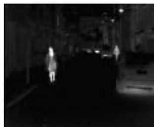
Photo 2. Image of FIR camera (pedestrians walking in front of the automobile)
