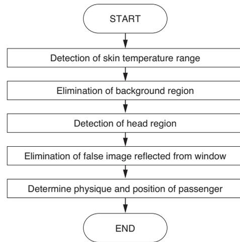
Fig. 9. Flowchart of the passenger detection algorithm
