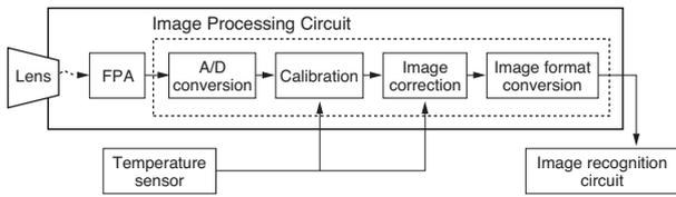
Fig. 8. Block diagram of the image processing circuit
