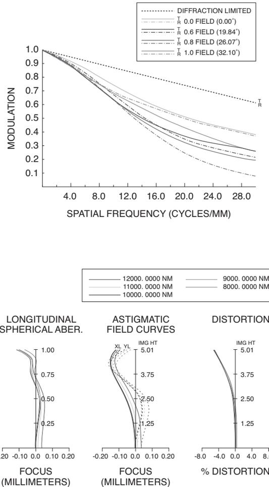
Fig. 3. MTF property and aberration diagram for the designed lens
