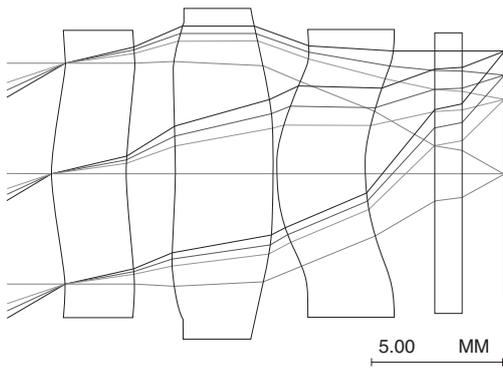
Fig. 2. Ray diagram for the designed lens
