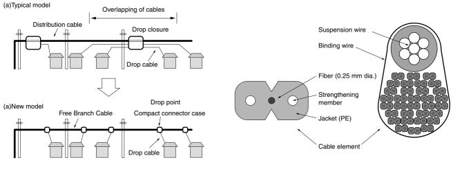
Fig. 1. Typical FTTH network model in Japan and new model
