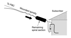
Fig. 8. Installation method for spiral drop cable
