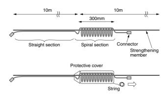
Fig. 7. Structure of spiral drop cable
