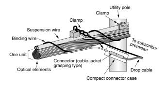
Fig. 3. Configuration of cable drop point
