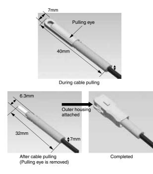
Fig. 9. Structure of slim connector
