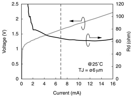
**Fig. 5.** Voltage-current (V-I) and current-differential resistance (Rd-I) characteristics of GaInNAs BTJ-VCSEL with 6- $\mu\text{m}$  diameter tunnel junction at 25°C
