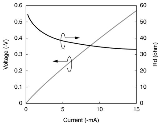
Fig. 2. Voltage-current (V-I) and current-differential resistance (I-Rd) characteristics of test structure
