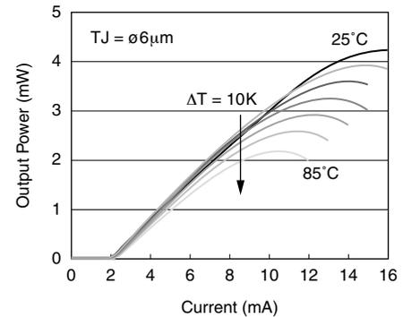
Fig. 3. Temperature dependence of light-current (L-I) characteristics of GaInNAs BTJ-VCSEL with 6- $\mu\text{m}$  diameter tunnel junction aperture
