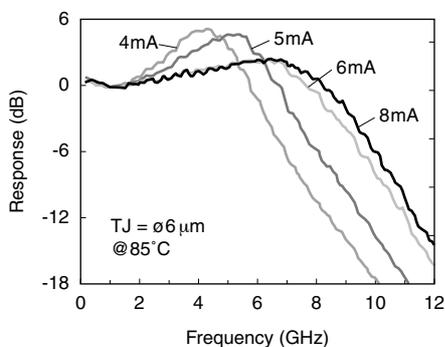
**Fig. 6.** Small signal responsiveness of GaInNAs BTJ-VCSEL with 6- $\mu\text{m}$  tunnel junction aperture at 85°C
