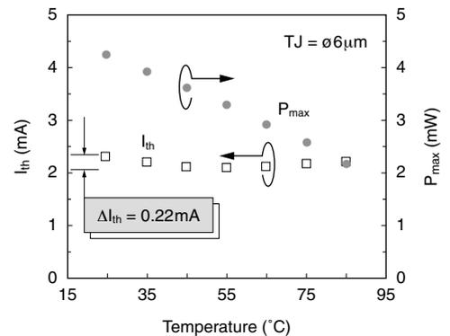
Fig. 4. Temperature dependence of threshold current and maximum output power of GaInNAs BTJ-VCSEL with 6- $\mu\text{m}$  diameter tunnel junction aperture
