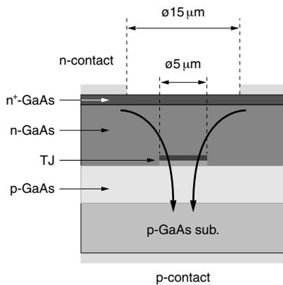
Fig. 1. Schematic diagram of BTJ test structure
