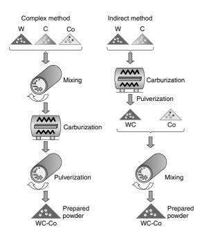
Fig. 2. WC-Co powder preparation methods (Complex method and indirect method)
