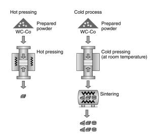
Fig. 3. Cemented carbide manufacturing methods (Hot pressing and cold process)
