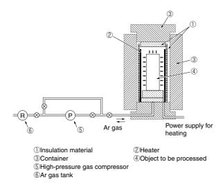
Fig. 6. Schematic view of HIP system
