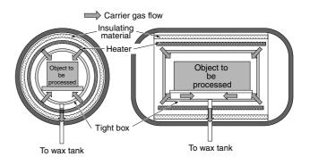
Fig. 5. Tight box structures
