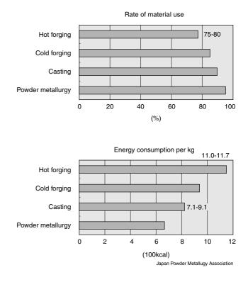
Fig. 1. Material use rate and energy consumption in different metal manufacturing methods
