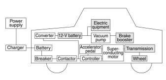
Fig. 6. Configuration of superconducting car
