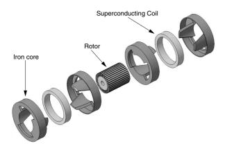
Fig. 3. Components of superconducting motor
