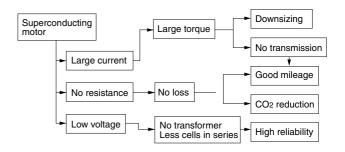
Fig. 1. Features of superconductor motor
