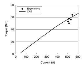
Fig. 5. Torque curve of superconducting motor
