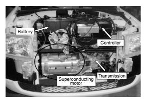
Photo 2. Superconducting motor fitted inside vehicle
