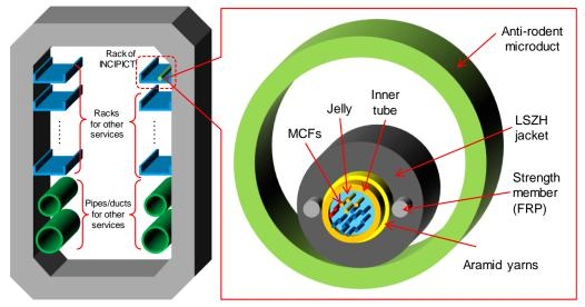
Figure 1: Schematics of the walkable underground tunnel with INCIPICT's rack (left), and the installed MCF cable in a microduct (right)
