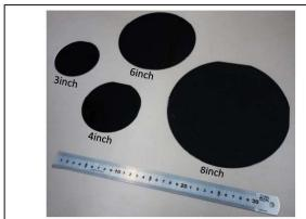
Fig. 1 Picture of 3-inch, 4-inch, 6-inch and 8-inch GaAs substrates.
