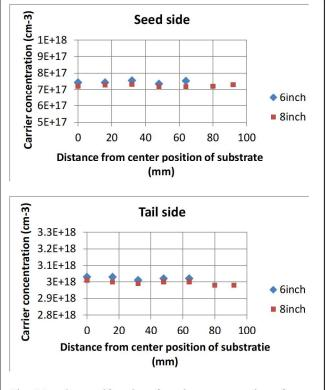
Fig. 5 In-plane uniformity of carrier concentration of GaAs substrates
