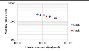
Fig. 6 The correlation between carrier concentration and mobility of 8-inch and 6-inch GaAs substrates.
