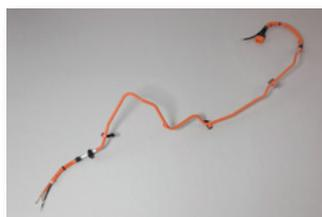
High-voltage wiring harness for HEVs
