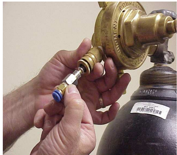
Figure 6 8mm Tubing Adapter Installed to Pressure Regulator
