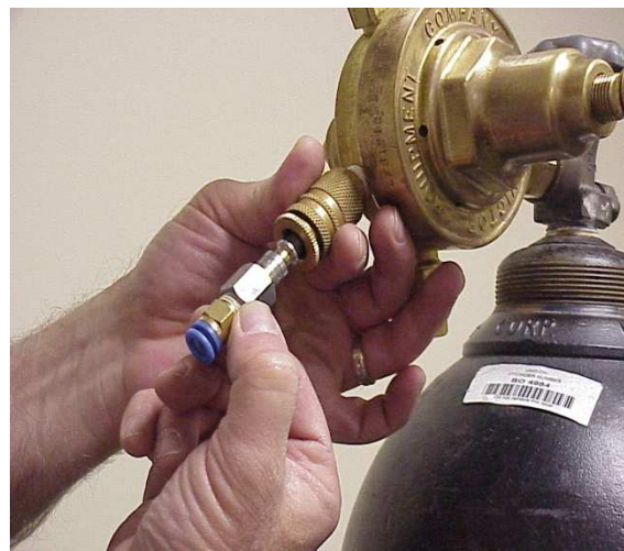
Figure 3 8mm Tubing Adapter Installed to Pressure Regulator
